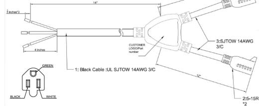
Material ......SJTOW Cable, polymeric splitter and connectors
