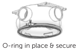
O-ring in place & secure
